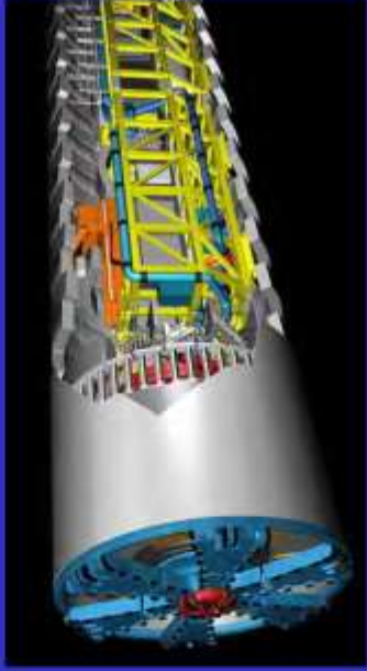
Tunnel Boring Machine (TBM)
